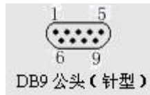
Figure 4. RS232 Pin Definition(Male/Needle Type)
