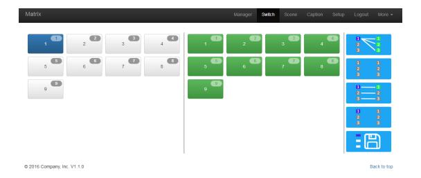
The left side of the long string is input area: Mini99 will have 9 buttons, Mini1818 has 18 buttons, Mini3636 will have 36 buttons. The right side is output area, the buttons are the same with input area. And there're 5 buttons: The 1<sup>st</sup> for 1 to all, 2<sup>nd</sup> for 1 off to all, 3<sup>rd</sup> for 1 to 1, 4<sup>th</sup> for all off, the last one is for scene save and recall. (Change names can be done in Caption interface)
