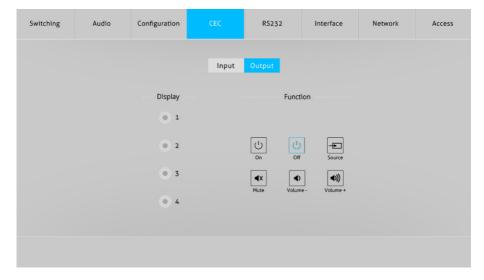
Select one output device to be controlled, and then press function buttons.
