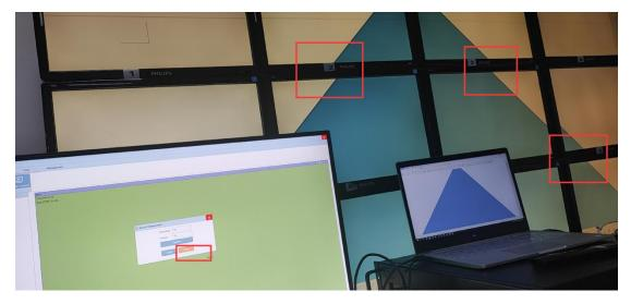
When with bezel correction or correction ON, it will be showing as below:
