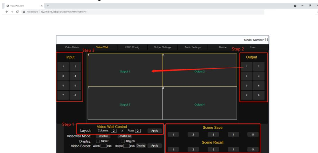
Video Wall box edge in yellow color means that outputs to this VW are all confirmed(use the mouse right click to confirm after drag the outputs)
