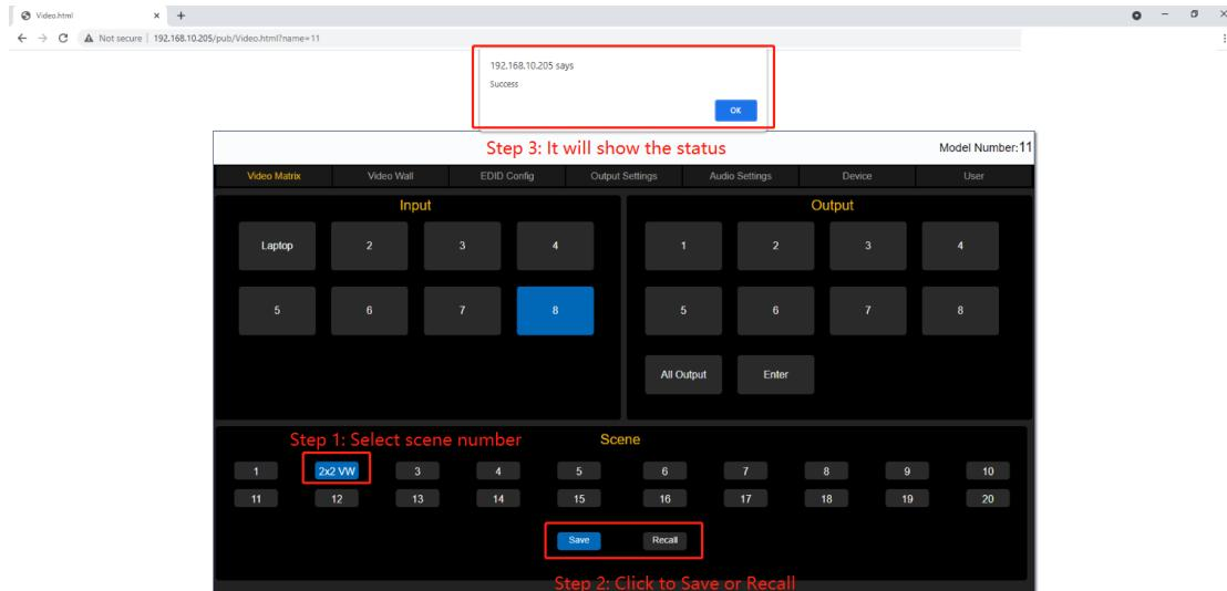
**Video Wall:** users can setup the VW wall, adjust the bezel, VW resolution, or save/recall the VW scenes:
